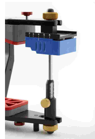
Gamma Sequence Incisal Table Condylography values used for calculations Protrusion at 5 mm: SCI 57.4° Mediotrusion right at 5 mm: SCI 63.7° TCI 14.5° Mediotrusion left at 5 mm: SCI 52.9° TCI -2.7° Suggested sequence table setting Protrusion element: ORANGE(YELLOW) Right lateral element: ORANGE(YELLOW) Left lateral element: ORANGE(YELLOW)
