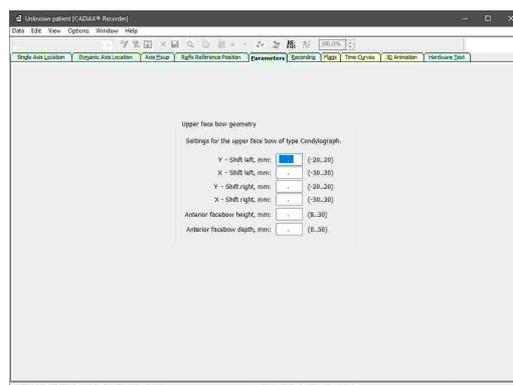
**Y-Shift** is the shift of either side arm of the upper bow to left or right side. It can be read from the scales on the front of the face bow's cross bar. Values that are located towards the inner side, relative to the zero point of the scale, are entered as negative values.
