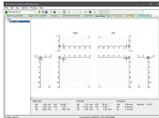
You can use the menu item *Data* → *Delete* or the corresponding toolbar button to remove an already performed recording.
