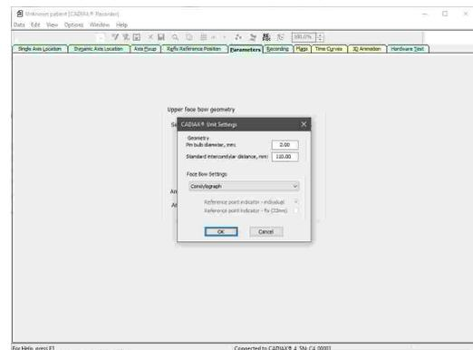
**STOP** The various face bows have different scales for entering face geometries. If a wrong face bow is selected or a wrong scale value is entered, the recordings can not be recalculated correctly. This can lead to a distorted picture of the recorded condylar tracks and, in some circumstances, to a falsification of the calculated value settings for the articulator.
