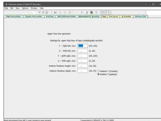
**Y-Shift** is the shift of either side arm of the upper bow to left or right side. It can be read from the scales on the top side of the face bow's cross bar.
