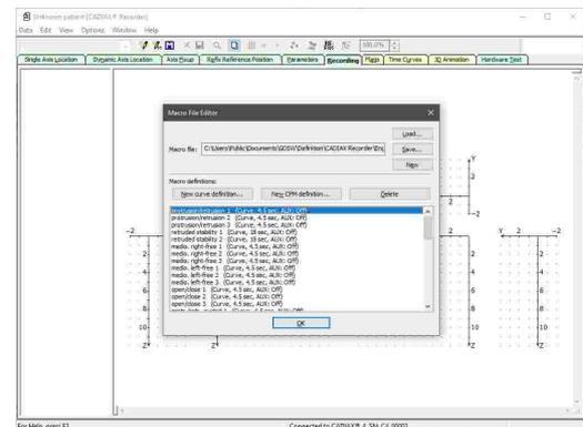
Use the provided buttons to add curve or CPM recordings to the sequence or to remove them. You can change the order of the items in the list by dragging them while holding the left mouse button. Once finished, save the macro to a file using the corresponding button.
