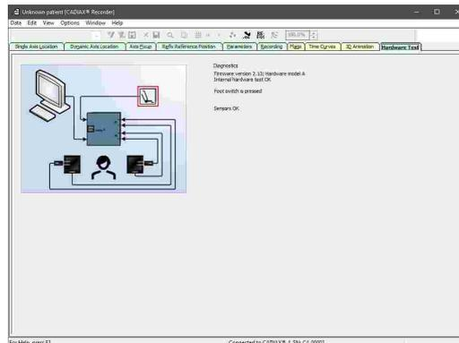
The display indicates errors in the system by highlighting the affected component in the graphic and shows an error description in the area *Diagnostics*.
