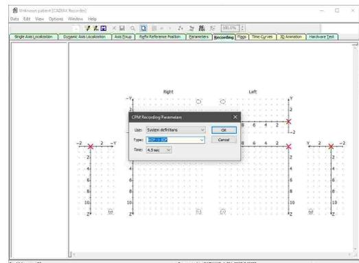
Similar to the curve recording parameters, **Type** is the name assigned to the CPM. A recording of type *Point Mode* can hold an unlimited number of individual point measurements, which are taken by pressing the foot switch repeatedly.
