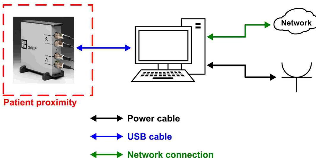
If such a computer is set up inside the patient's proximity, it and all devices connected to it (e.g. monitor) have to be isolated according to EN 60601-1. Power sources have to be connected through a medical isolation transformer and tethered network connections through a medical network isolator.
