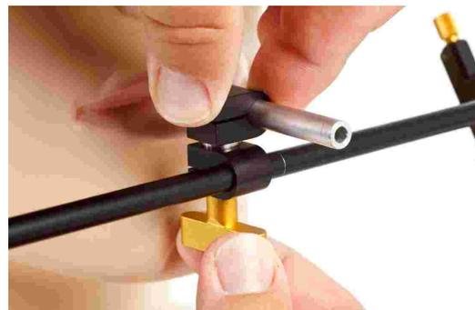
Insert the axis needles into the retainers at the end of the side arms and adjust their location to the approximate position of the joint axis.
