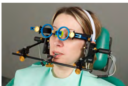
The condylograph carries the measurement sensory system used in the CADIAX ® 4 system
