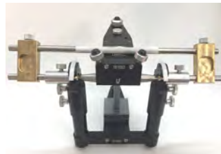
Connect the condyle bars with adjustment adhesive again by using the adjustment tool and the Reference Calibration key
