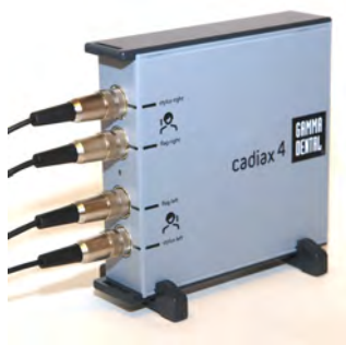
The CADIAX 4 device with the "diagnostic" sensor set connected, which occupies all four of the device's connectors.
