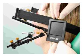
Fixate the styli with the respective screws in the retainers of the lower face bow. The cable of the stylus should hang downwards after it is fixated.
